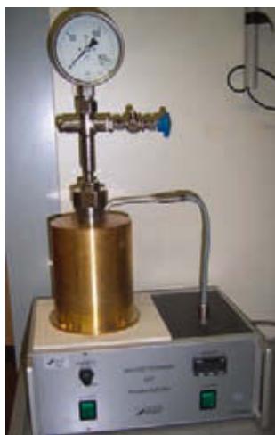
Picture 19a: Manual autoclave with hotplate stirrer
