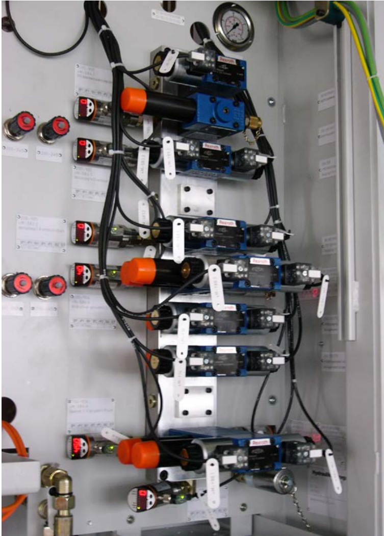
Fig. 20 Marking hydraulic valve blocks
