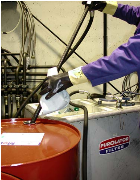
Fig. 5 Personal protective equipment for oil change
