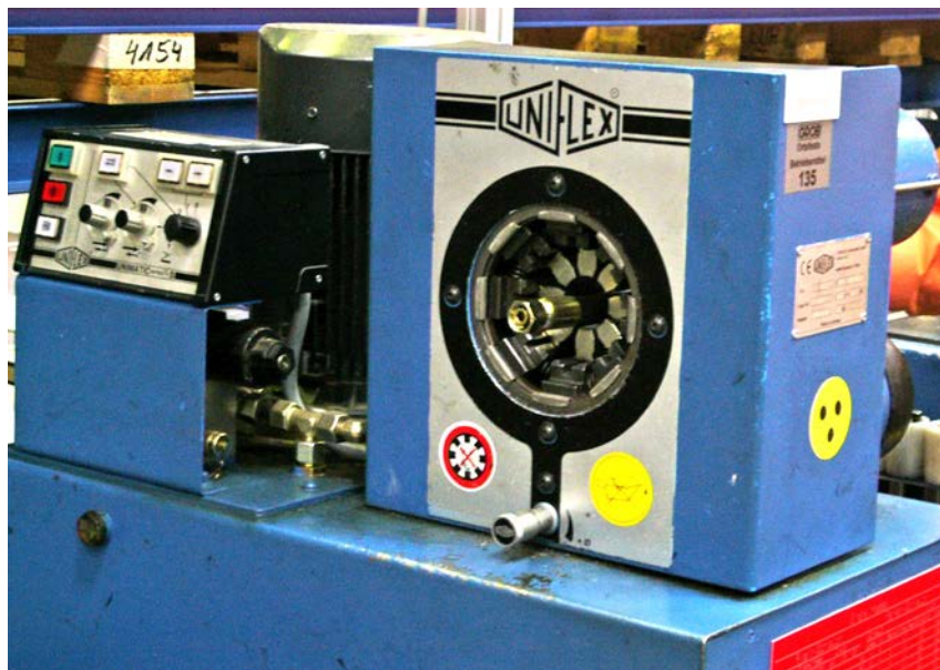
Fig. 14 Device for pressing hose fittings
