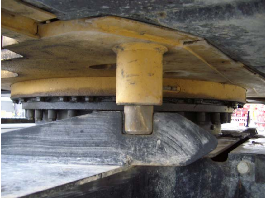
Fig. 40 Swivel lock on a hydraulic excavator in locked position
