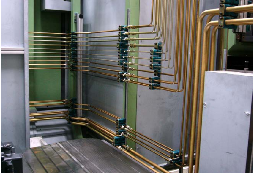
Fig. 10 Proper attachment of pipelines with pipe supports
