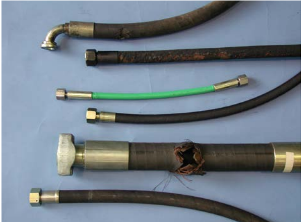
Fig. 16 Examples of failed hydraulic hose assemblies
