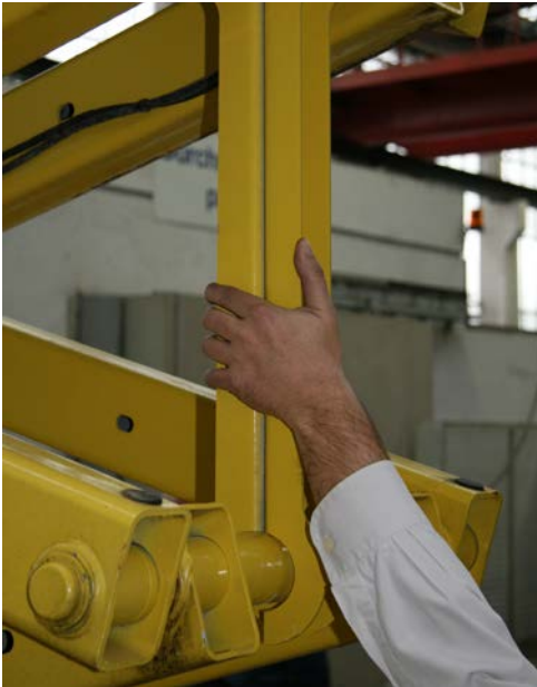
Fig. 29 Installed maintenance support on hydraulic scissors lift
