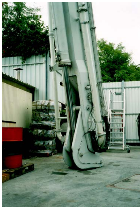
Fig. 38 Boom of a concrete pump lowered to the ground
