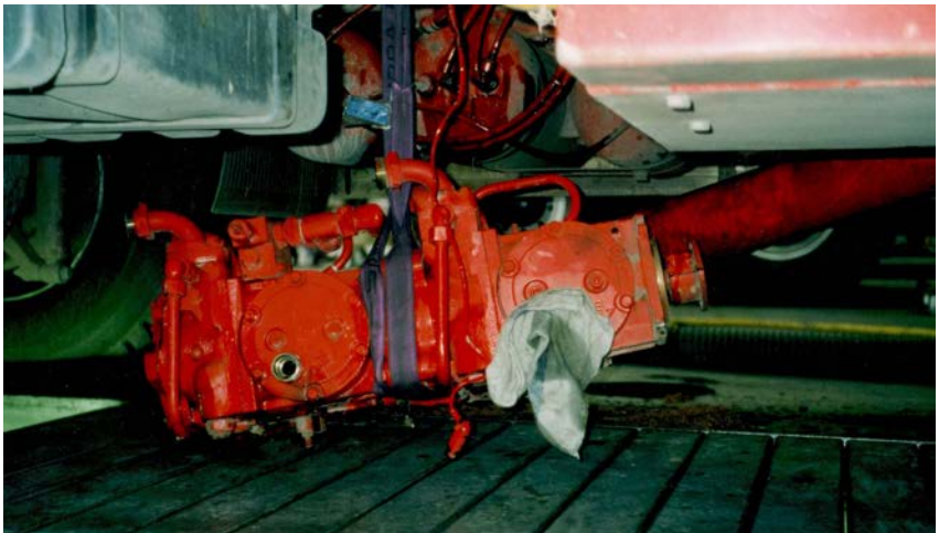
Fig. 39 Vehicle main pump on a load lifting device
