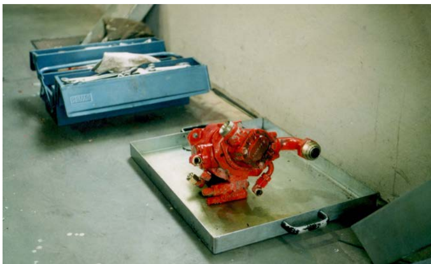
Fig. 19 Mobile hydraulic pump in an oil drip pan
