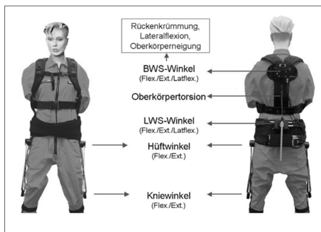
Abbildung 21: Messsystem CUELA (Basisversion); BWS = Brustwirbelsäule, LWS = Lendenwirbelsäule; Flex. = Flexion; Ext. = Extension; Latflex. = Lateralflexion
