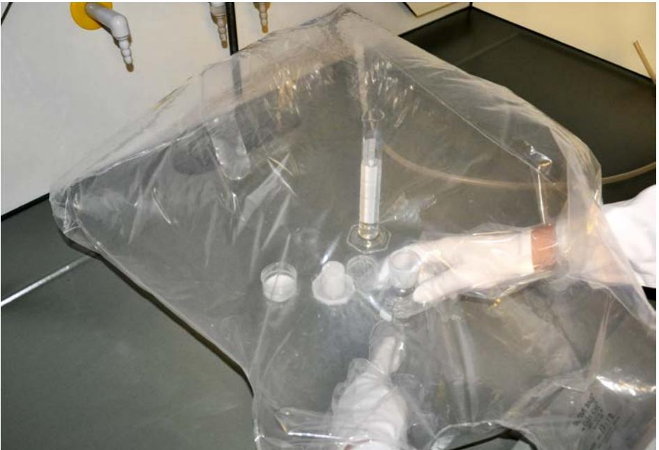
Fig. 14 Glove bag with closing clip for feed opening
