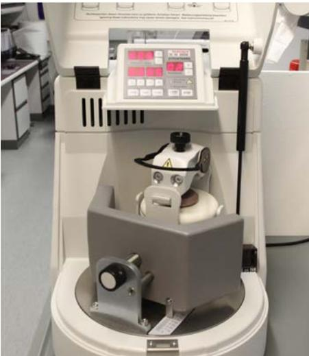
Fig. 10 Ball mill with closed grinding bowl
