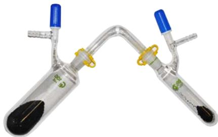
Fig. 6 Transfer bow for powders protected from draughts (if necessary inert gas – Ar to be preferred – can be used to protect the powder against moisture and air)
