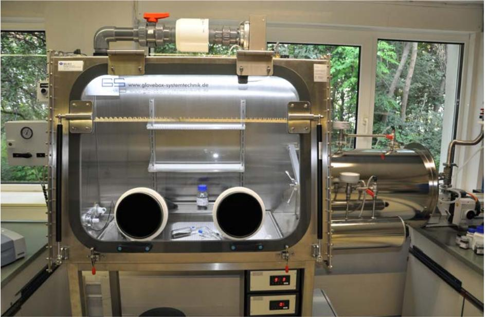
Fig. 13 Glove box with airlock
