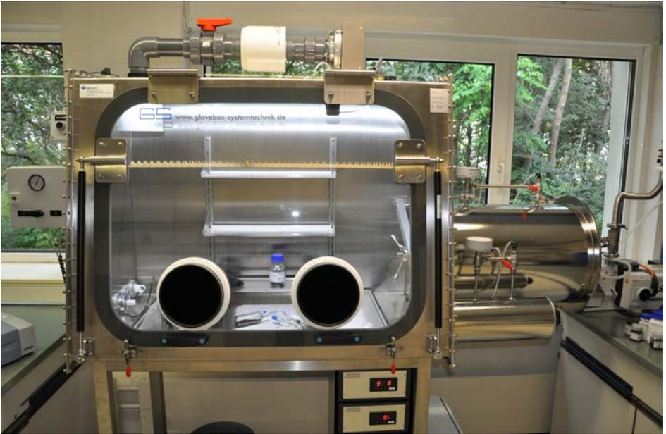
Fig. 13 Glove box with airlock
