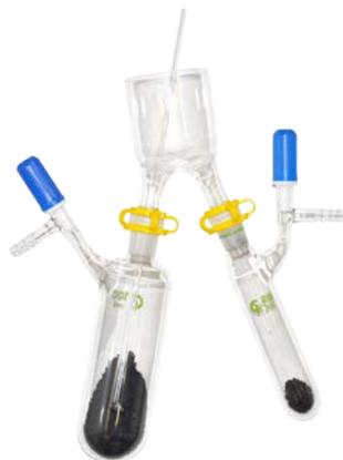
Fig. 7 Transfer with a glass spatula protected from draughts (if necessary inert gas – Ar to be preferred – can be used to protect the powder against moisture and air)
