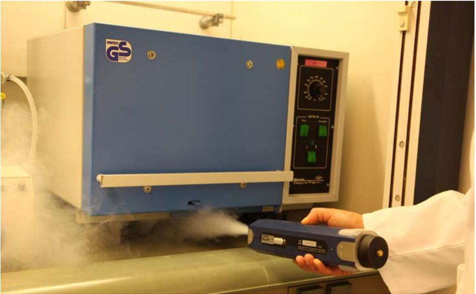
Fig. 4 Testing the fume hood with a smoke generator
