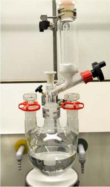
Fig. 8 Manual powder dosing funnel on a three-necked flask
