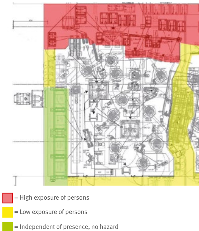
Fig. 39 Example of a system safety layout [J]
