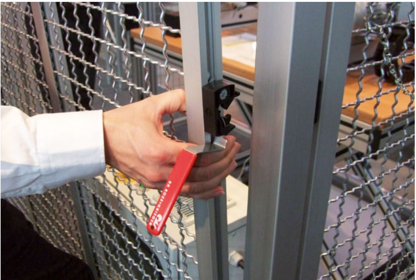
Fig. 37 Fixtures remain connected to the protective devices or to the machine after removing the protective devices (example). [H]
