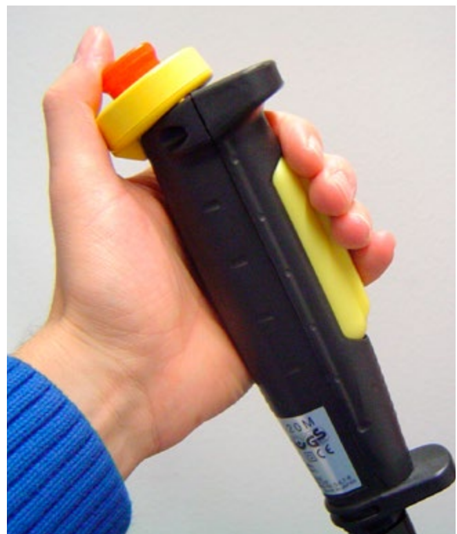
Fig. 55 Enabling switch during trouble-shooting [H]
