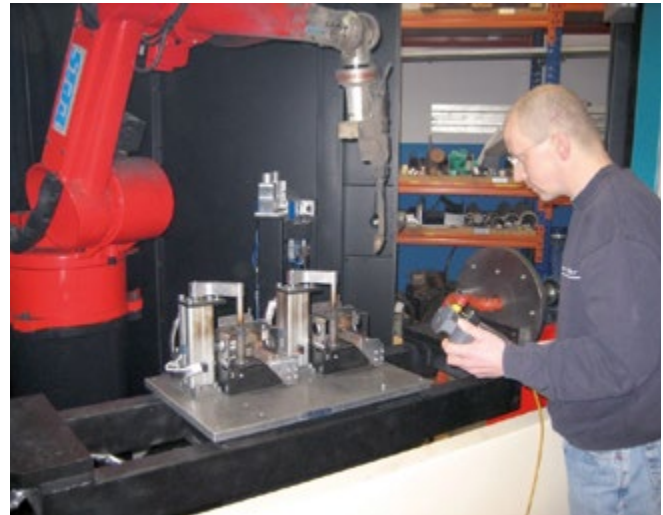
Fig. 28 Actuation of the enabling switch during programming [F]
