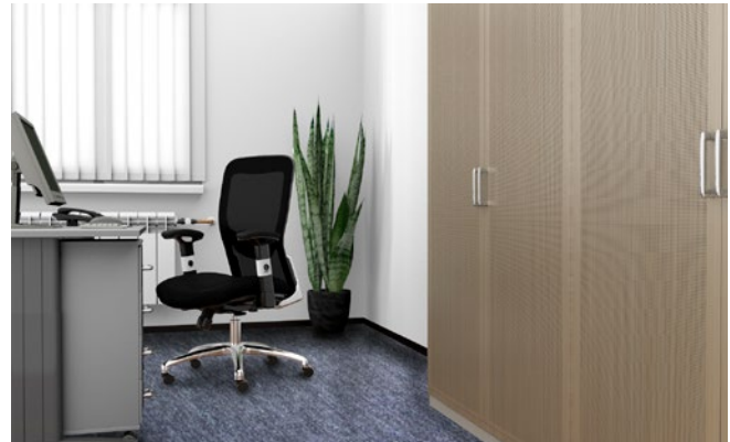
Figure 5 Means of improving room acoustics: Sound-absorbent vertical slat blinds, furniture with sound-absorbent surfaces, sound-absorbent carpets
