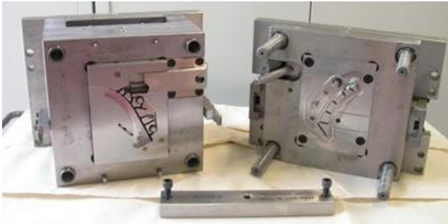
Figure 1 – Mould halves of an injection mould
