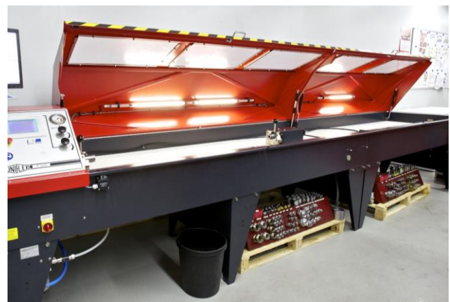
Figure 2: Pressure- und leak tightness test bench for hydraulic hoses with guard open
