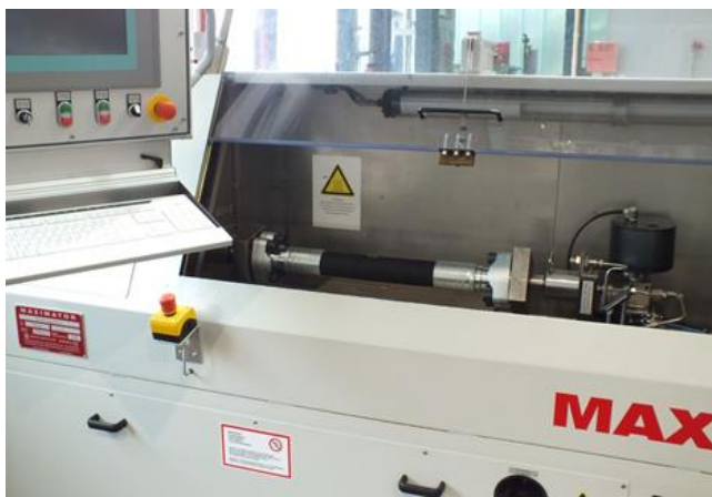
Figure 1: Burst pressure test bench with guard open
