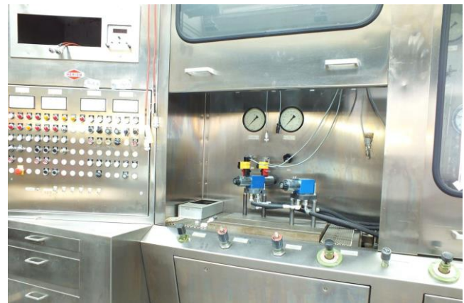
Figure 3: Hydraulic component test bench with guard open
