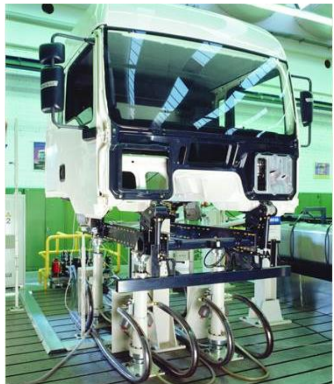
Figure 9: Servo cylinder for highly dynamic simulation of movements in a separate test room
