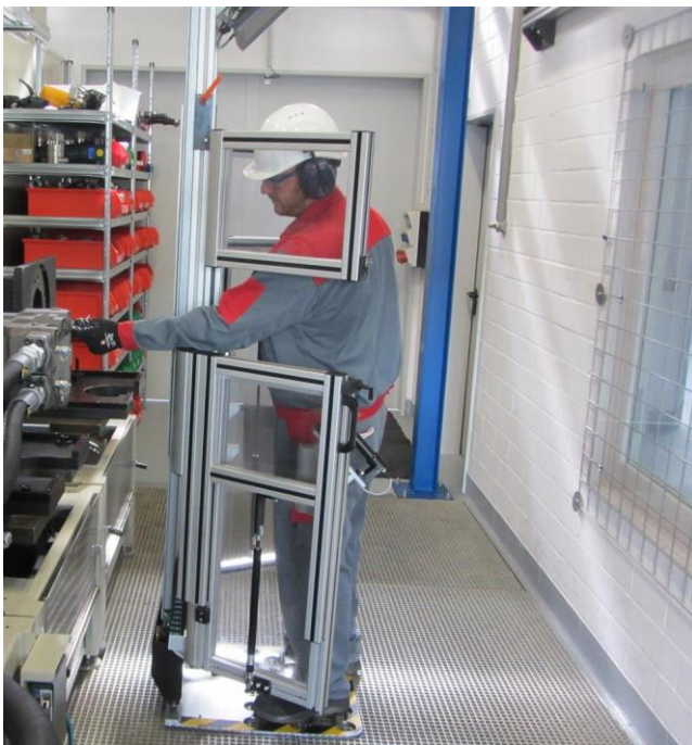
Figure 7: Manually adjustable protective device for maximum protection during the adjustment on a pump test bench in a separate test room
