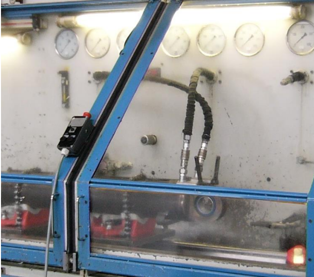
Figure 5: Hydraulic cylinder test bench with closed guard
