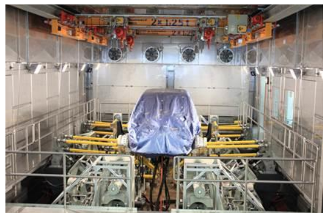
Figure 8: Servo hydraulic chassis test bench in a separate test room
