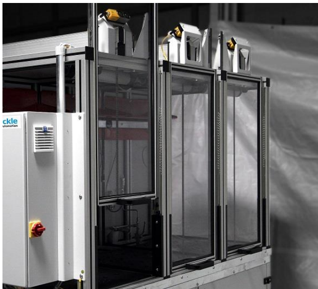
Figure 6: Open guard on a hydraulic test bench
