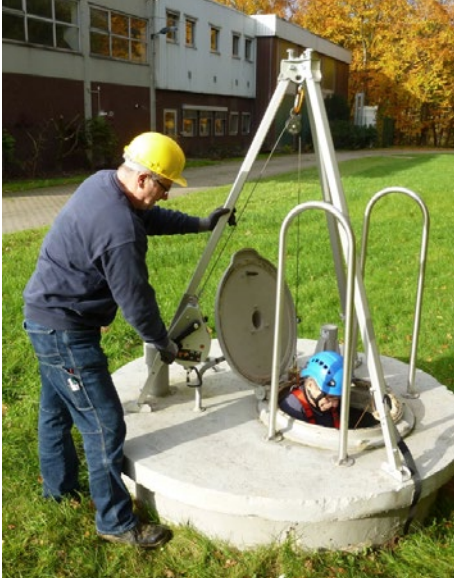
Fig. 27 Rescue by means of a fall arresting device with rescue lift function
