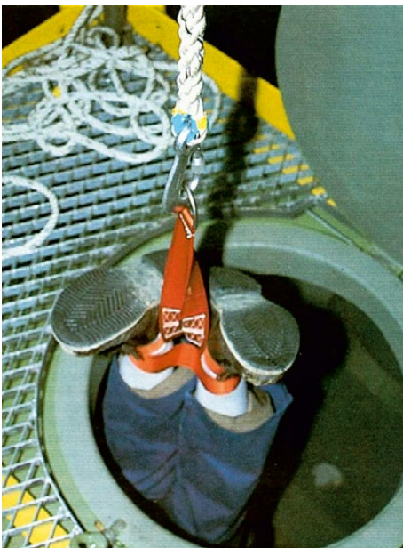
Fig. 28 Rescue sling (particularly suitable for fast rescue, for example where the person to be rescued is not wearing a full body harness, and risk to life is presented by an oxygen deficit or hazardous substances)
