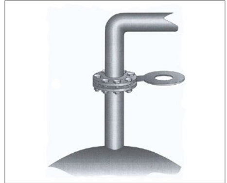
Fig. 18 Isolation by means of a sealing blank
