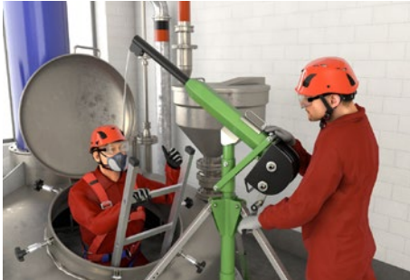
Fig. 22 Rescue winch, being used in this case for protection against falling
