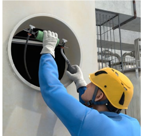
Fig. 20 Sampling by means of a gas sampling tube
