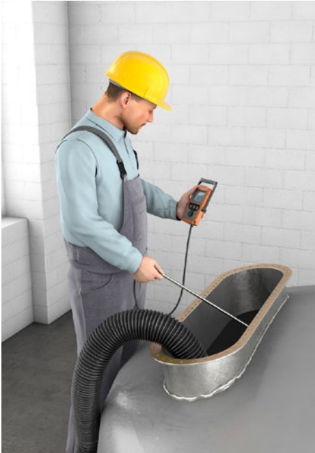
Fig. 19 Sampling by means of gas measuring instruments
