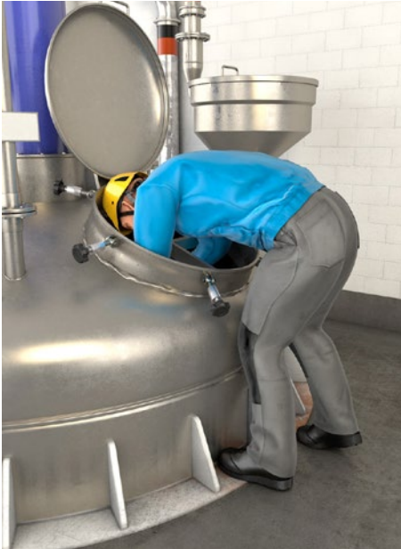
Fig. 3 Inspection tasks (leaning into the vessel or confined space): permissible only with additional protective measures. In this case: a protective mesh in the manhole that prevents persons from falling into it
