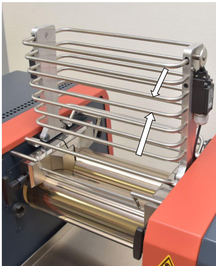
Fig. 4: Roll mill with rocker switch on the feed funnel and switch bracket on the roller
