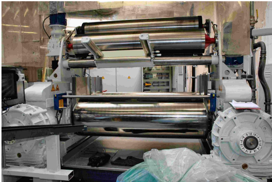
Fig. 3: Operating side of a roll mill with shift bar at 1400 mm height
