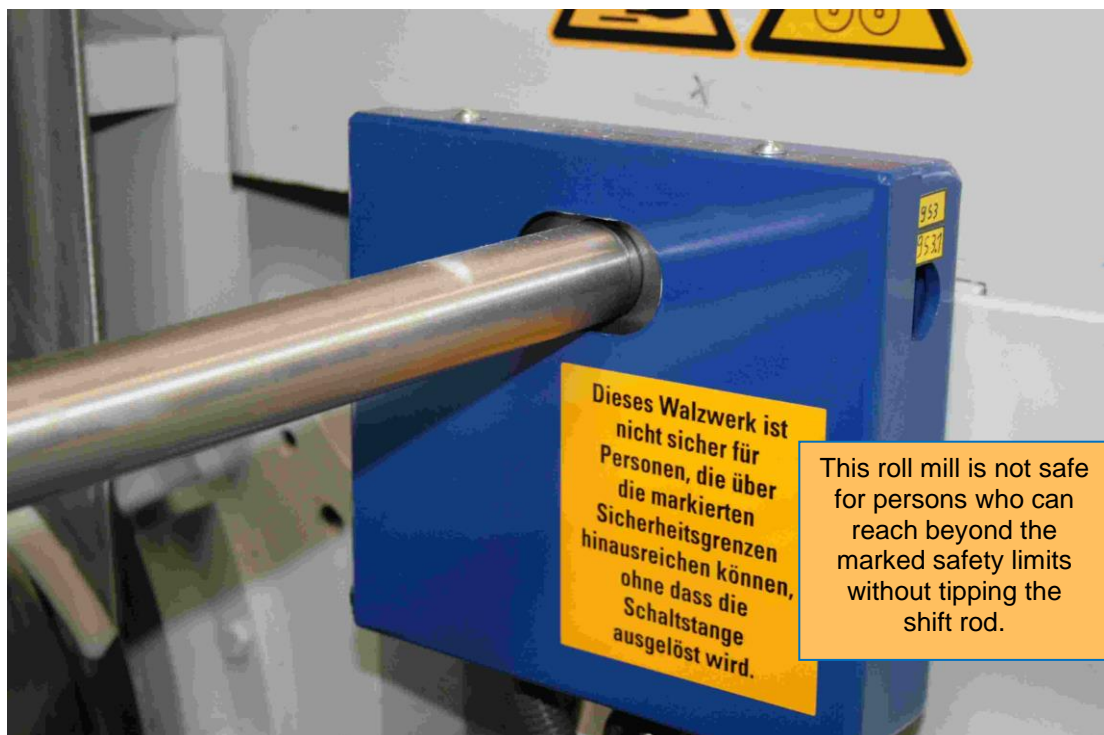
Fig. 4: Manipulation easily possible by clamping the shift rod
