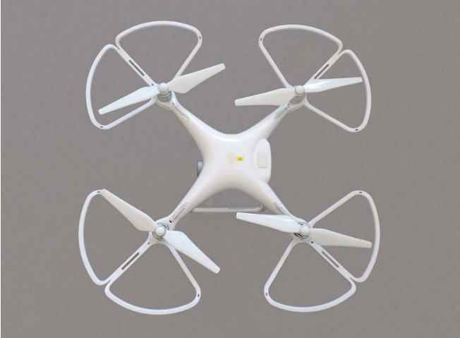
Abb. 8 Quadkopter in X- Bauform
