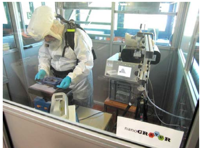
Test chamber for simulation of activities involving nanoparticle composites (image: IFA).
