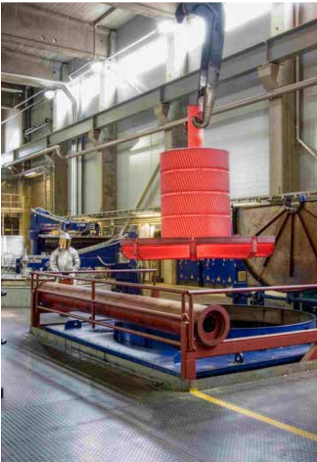
Figure 11 Red-hot charge on the crane (before quenching)
