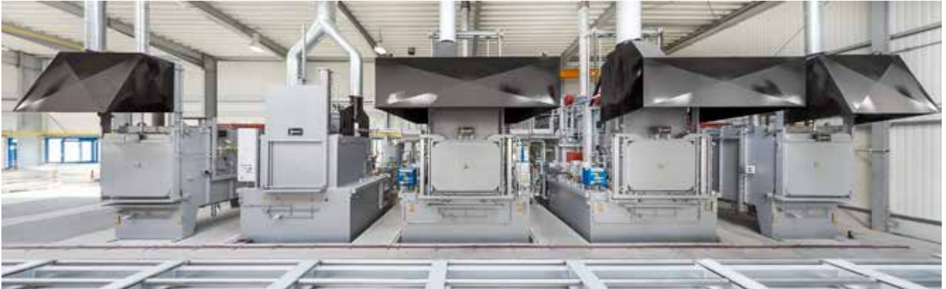
Figure 35 Installation comprising tempering furnace, cleaning plant, two hardening furnaces, tempering furnace
