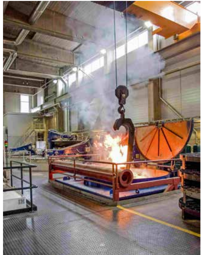
Figure 43 Charge immersed in an open oil bath
