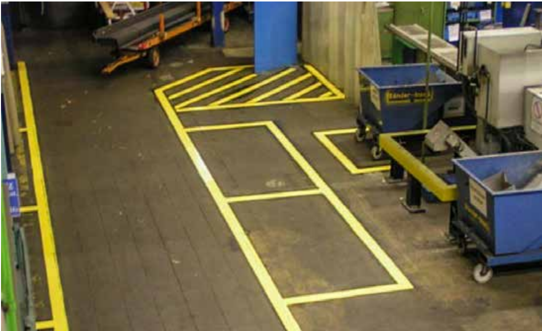
Figure 7 Marking of traffic routes, reception/staging areas and closed areas
