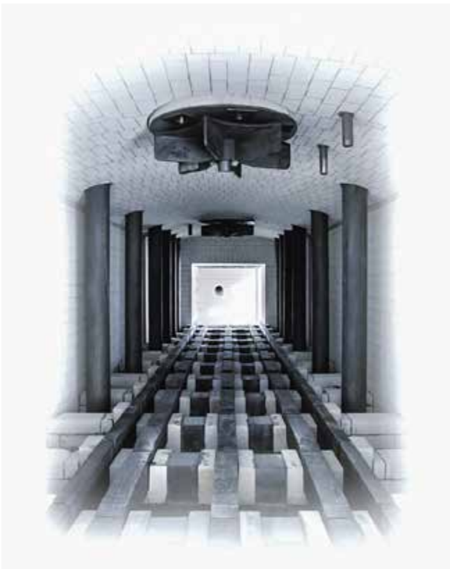
Figure 12 Furnace chamber in a pusher type furnace
