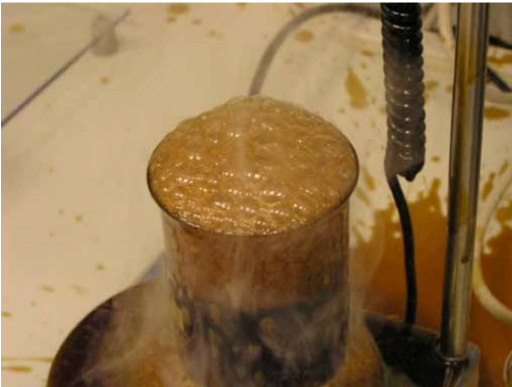
Figure 33 Oil foam formation on hardening oil contaminated with water (simulated in the laboratory)
