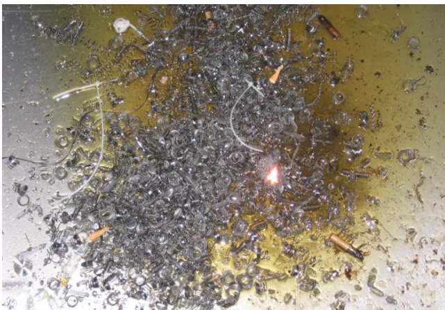
Figure 7: Ignition sources cigarette ends, fire in chip container
