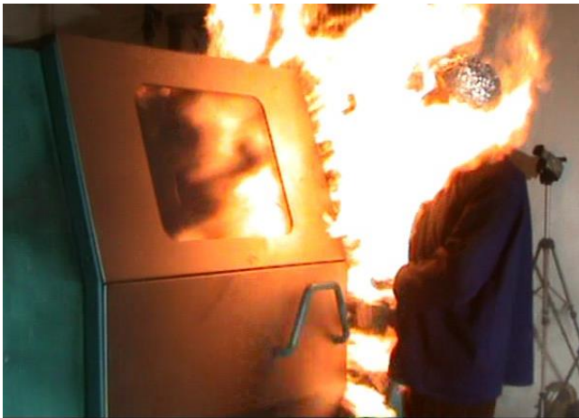
Figure 5: Flame ejection from open door gap (6 cm) during a deflagration (Dummy)
