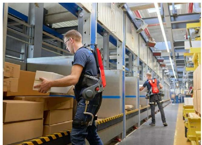
Abb. 2 Aktives Exoskelett Cray X, Foto: © German Bionic
