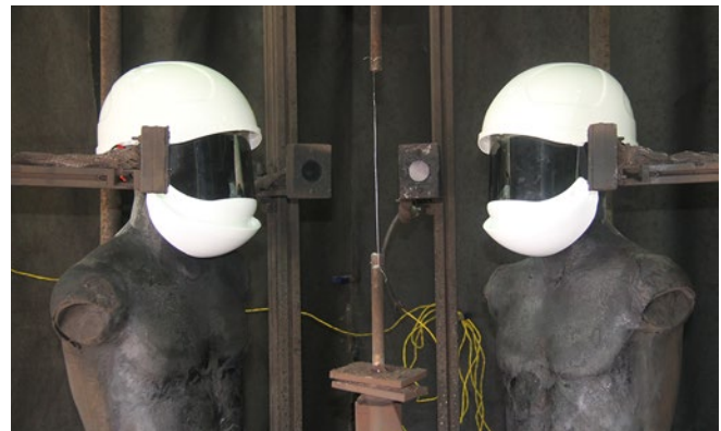
Fig. A 2-2 ATPV Test setup
