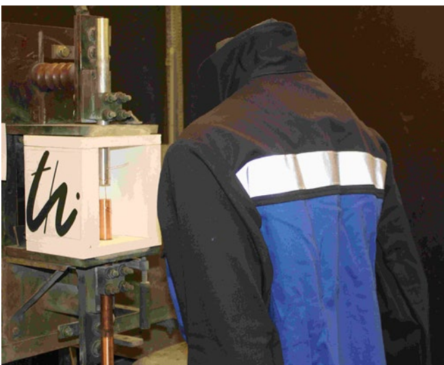
Fig. A 2-1 Test setup, Box test method
