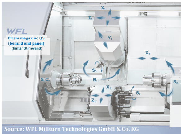
Figure 1: Diagram showing the axes of a machine tool
