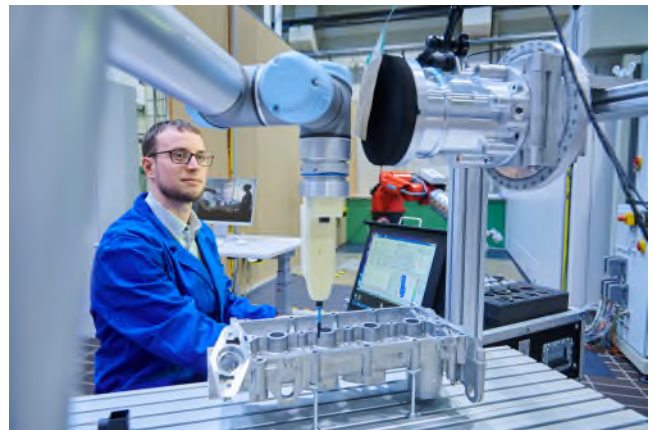
Testing the collision forces of a collaborative robot system
