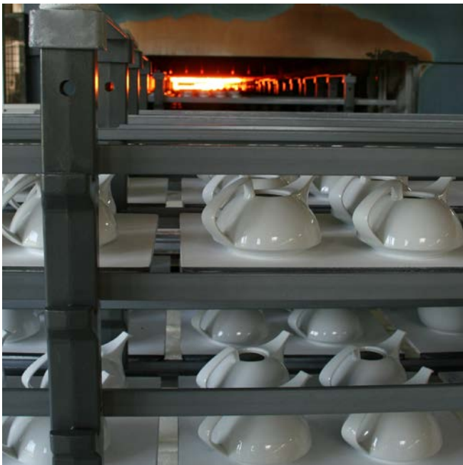
Figure 20: Glost firing of porcelain articles
