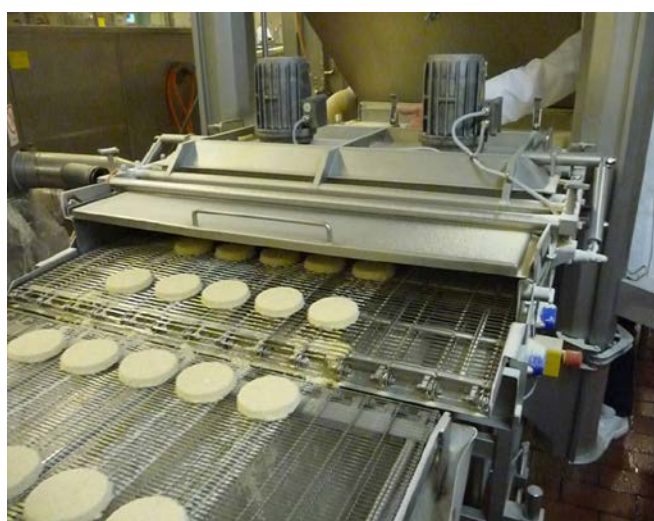
Figure 42: Breading of vegetable burgers: the product is first pressed into slices, after which it undergoes wet and dry breading. Dry breading not adhering to the product is blown off. This results in dry breading escaping from the machine into the surrounding work areas, despite the exhaust equipment and partial encapsulation. The same process is also used to bread fish, such as fishcakes or fish fingers, and in meat processing, for example for breading cutlets for the convenience foods sector.
