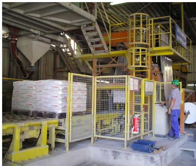
Figure 12: Packing and loading of ready-mixed plaster on pallets
