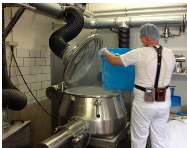
Figure 41: Weighing out of raw materials in powder form: various raw materials in powder form are weighed out on a scale with dust exhaust (not shown in the image) and then manually fed into the mixer. An exhaust hose is located to the right of the mixer; the lid of the mixer is also exhausted. A further exhaust facility is located at the outlet (bottom left).
