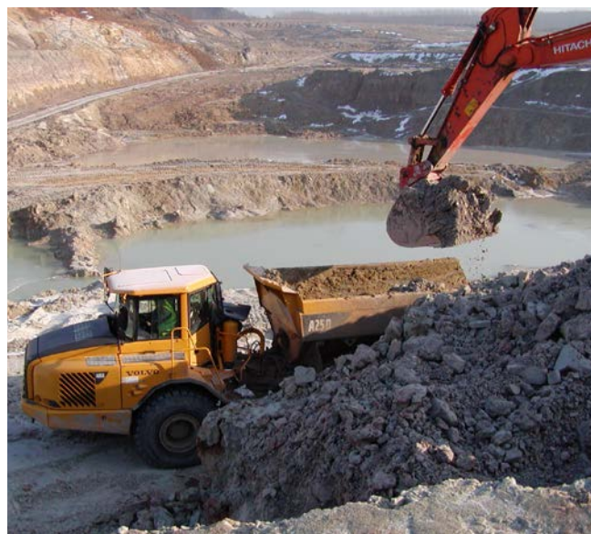
Figure 17: Extraction of kaolin in open-cast mining
