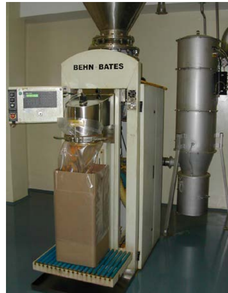
Figure 28: Filling station with exhaust equipment
