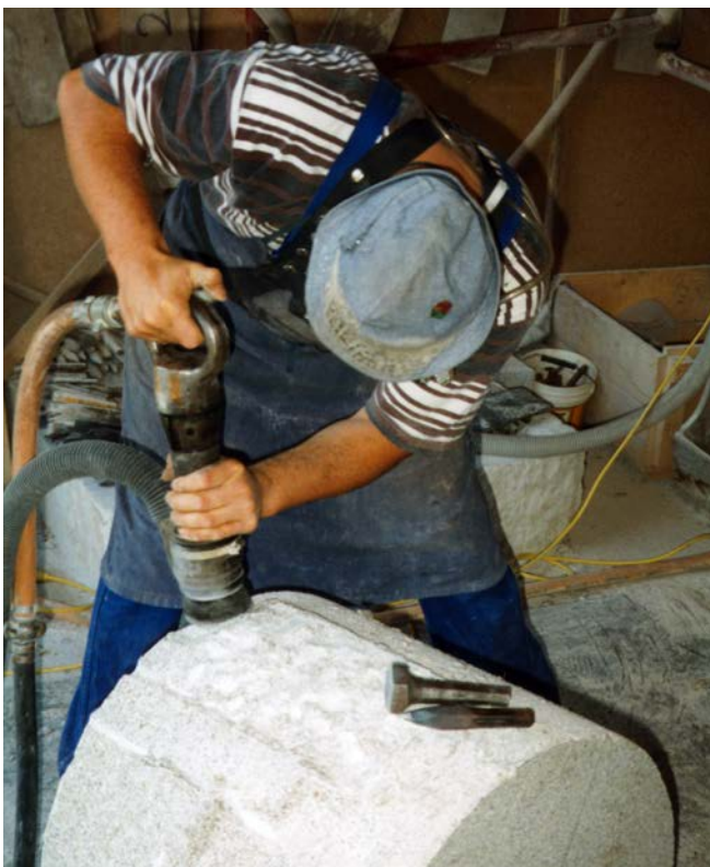
Figure 7: Manual working of natural cut stones: bush-hammering
