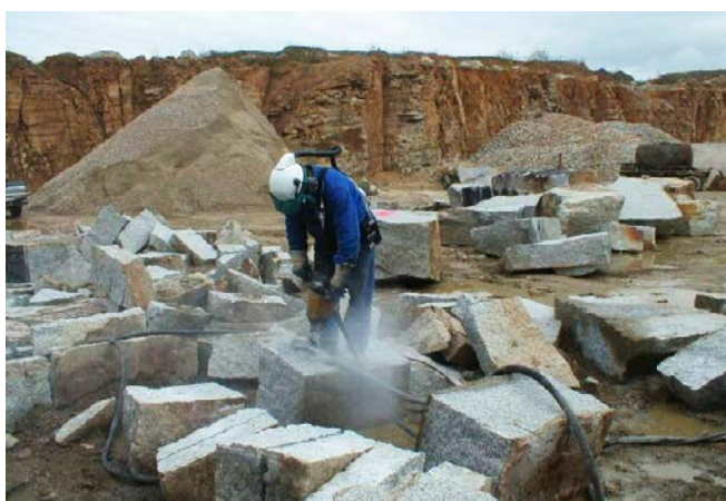
Figure 3: Use of a pneumatic hammer to split natural stone
