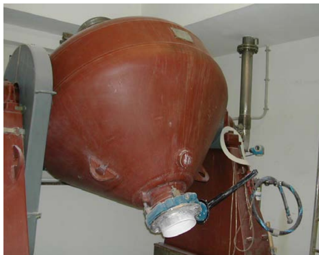
Figure 29: Mixing drum for the production of dry mixtures
