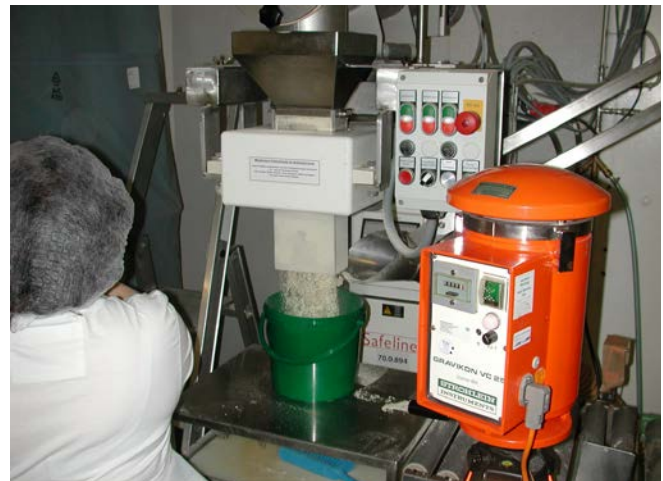
Figure 46: Semi-automatic filling of dry products such as soups, sauces, stock or seasoning for bulk consumers into tubs on a packaging line. Raised dust is exhausted in some cases through an exhaust funnel (to the right above the tub). The worker places the tubs in position, checks that they are filled correctly and closes the lid manually.
