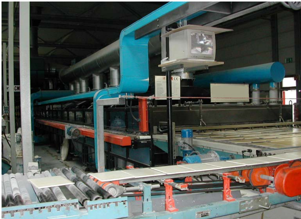
Figure 23: Tile production in a fast-firing kiln
