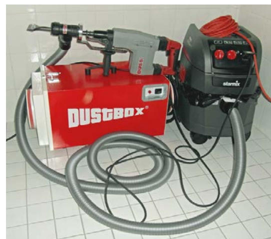
Figure 52: Power tool (in this case a demolition hammer) with dust exhaust, construction site dust collect and air purifier. Together with a dust-proof partition (not visible in the image), these comprise the basic equipment for low-dust working methods for each company.
