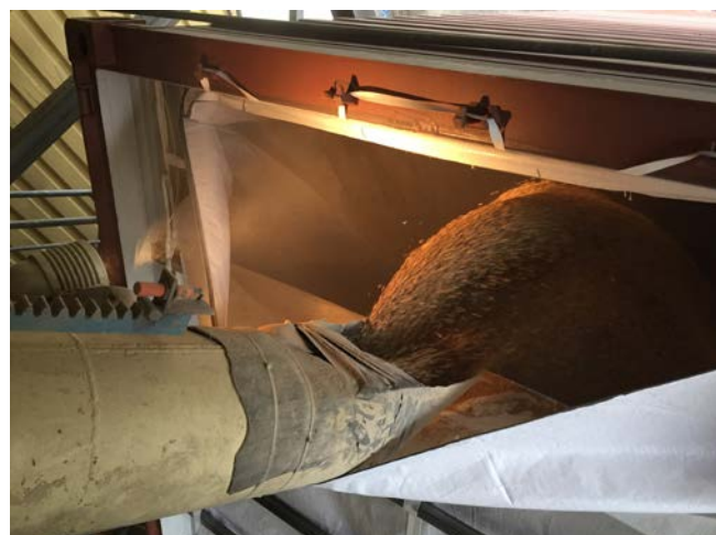
Figure 47: Filling a lined 20-foot container with brewer's malt in the partially encapsulated outdoor area. The product's drop height of up to several metres releases considerable quantities of dust. During filling, the entire truck and the container mounted on it is tilted on a platform by approximately 40°. One worker is present here intermittently to check correct filling and to take product samples for quality assurance.
