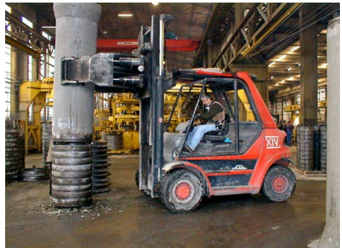
Figure 14: Pipe manufacture in the concrete industry
