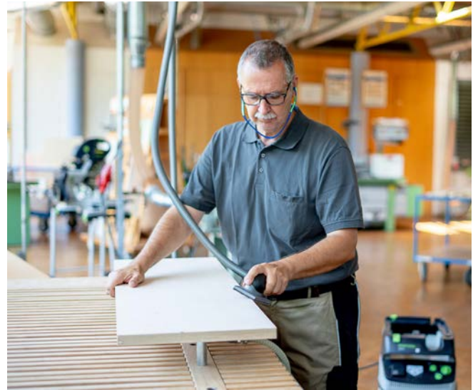
Figure 35: Manual sanding with a hand-held sanding block, with dust exhaust
