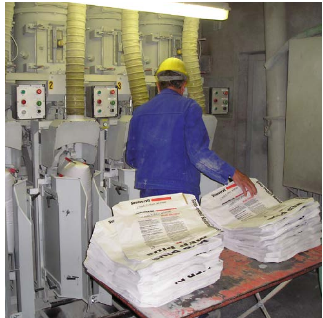
Figure 11: Bagging of ready-mixed plaster
