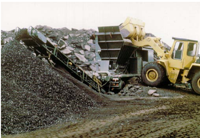
Figure 50: Charging of a crusher in construction material recycling
