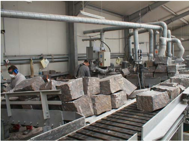
Figure 8: Mechanized splitting of stone blocks
