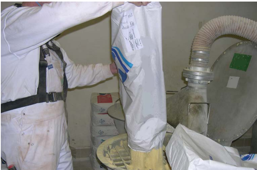
Figure 40: Loading a mixer: the worker adds various ingredients of the feed, supplied in bags, into the mixer. A vacuuming element is located behind the feed hopper
