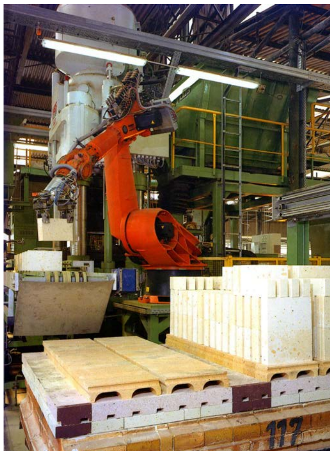
Figure 16: Placing of refractory products on kiln cars
