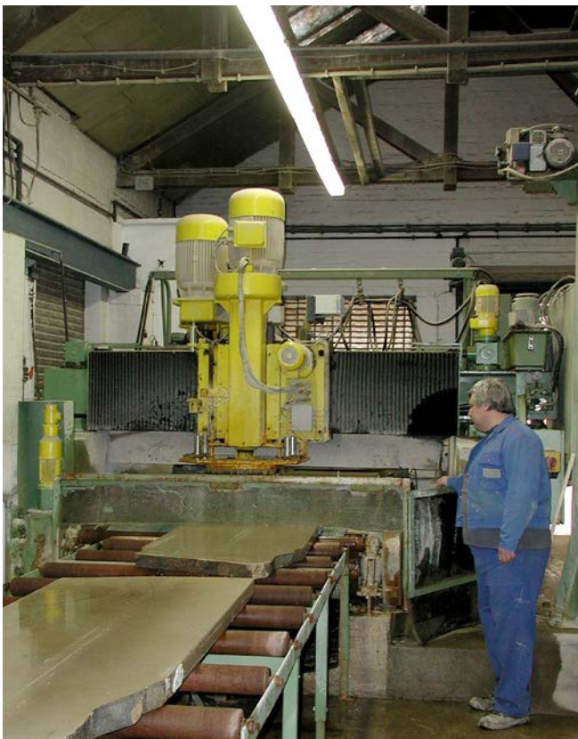
Figure 9: Mechanized wet grinding of natural cut stones
