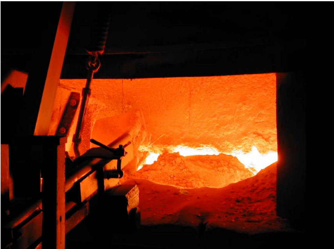
Figure 15: Loading of the batch into the tank
