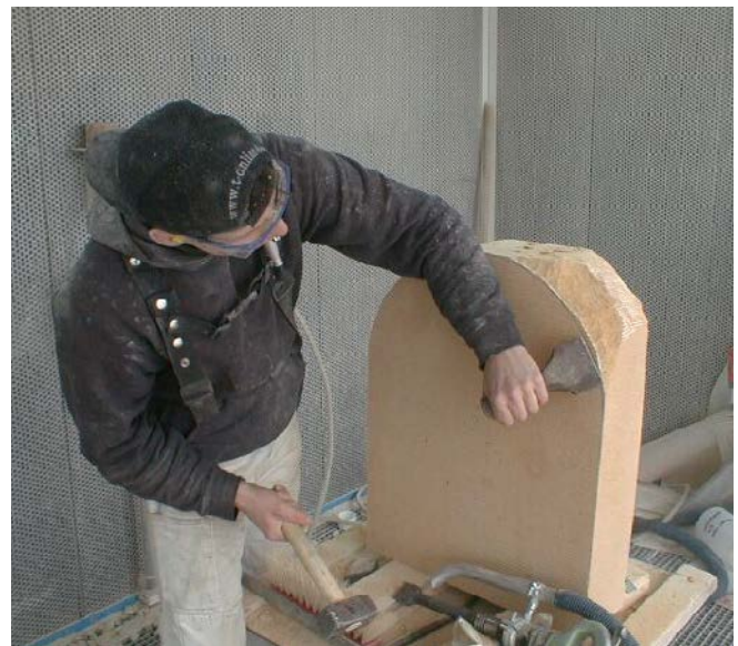
Figure 6: Manual working of natural cut stones: bossage
