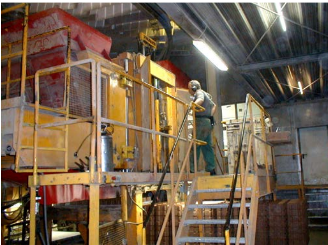
Figure 13: Concrete block machine
