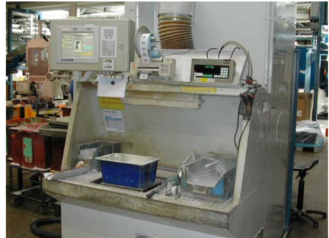
Figure 30: Weighing out and mixing station in the rubber industry
