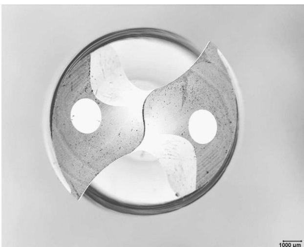
Figure 3 – Applied twist drills for dry machining in the front view
