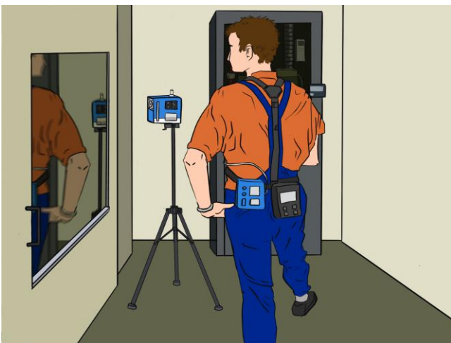
Figure 9 – Exposure measurements taken on the operator and stationary at the control panel
