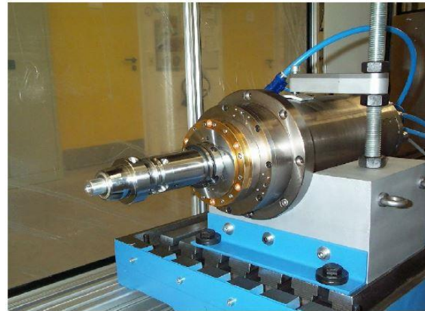
Figure 1 –Spindle test bench with HSC-motor spindle for internal aerosol supply
