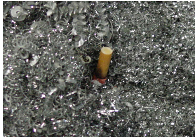
Figure 6 – Source of ignition in the chip container
