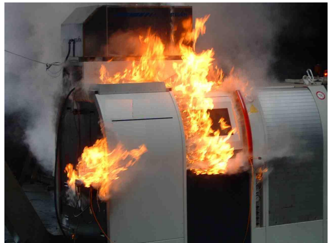
Figure 1 – Flame ejections on a machine tool after ignition of MWF-air mixture [1]
