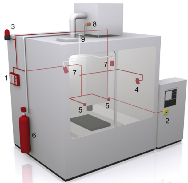
Figure 1 – Fire suppression system integrated into a machine tool
