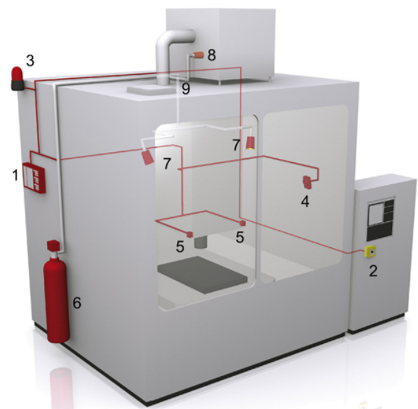
Figure 1 – Fire suppression system integrated into a machine tool
