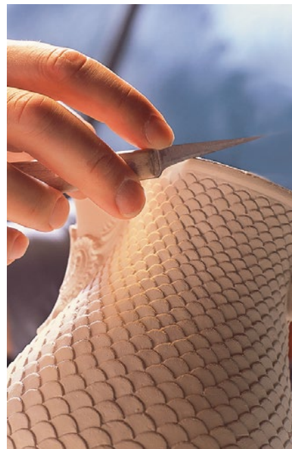
Figure 21: Manual white fettling of porcelain. Source: VBG
