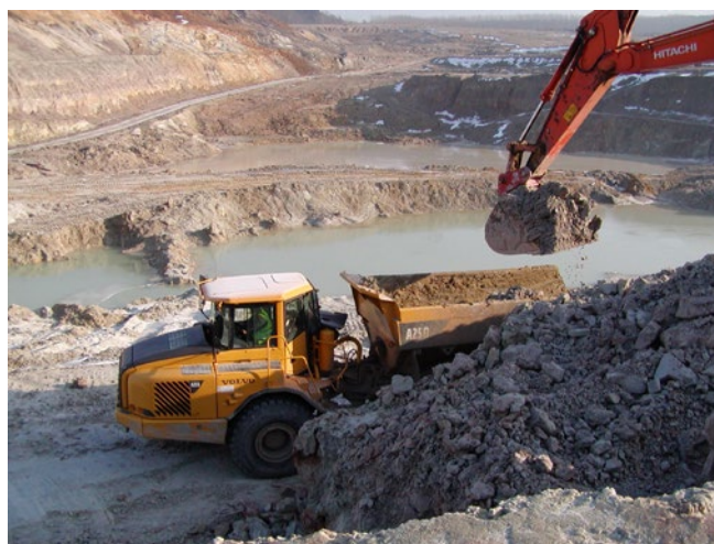
Figure 14: Extraction of kaolin in open-cast mining. Source: VBG
