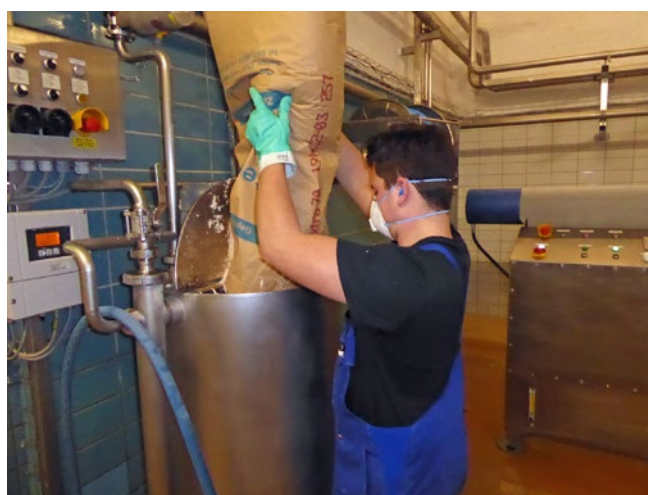
Figure 34: Filtration aids are added during beverage production. Source: BGN
