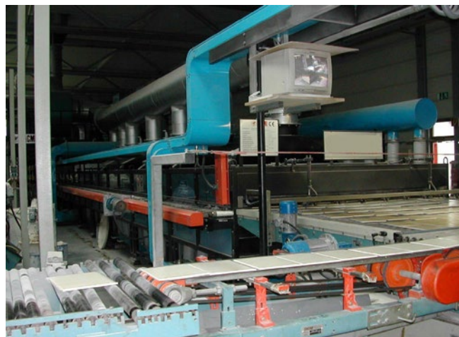
Figure 28: Tile removal behind a fast-fire tunnel kiln. Source: VBG
