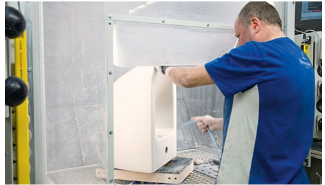
Figure 23: White rendering on WC basins in a white rendering cabin. Source: VBG
