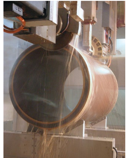
Figure 30: Wet grinding of vitrified clay pipes. Source: VBG
