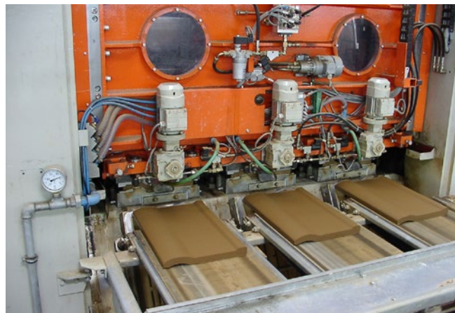
Figure 32: Roof tile after the pressing process on a turret. Source: VBG
