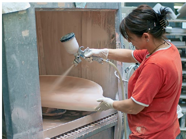
Figure 29: Spray glazing of tiles. Source: VBG
