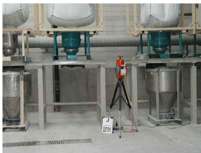
Figure 26: Low-dust feeding of raw materials using big bags. Source: VBG
