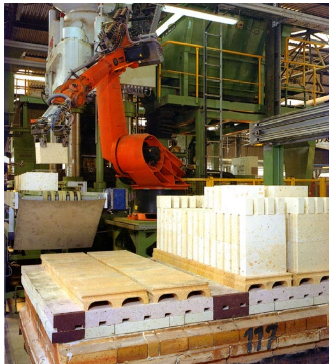
Figure 16: Placing refractory bricks on kiln cars. Source: VBG
