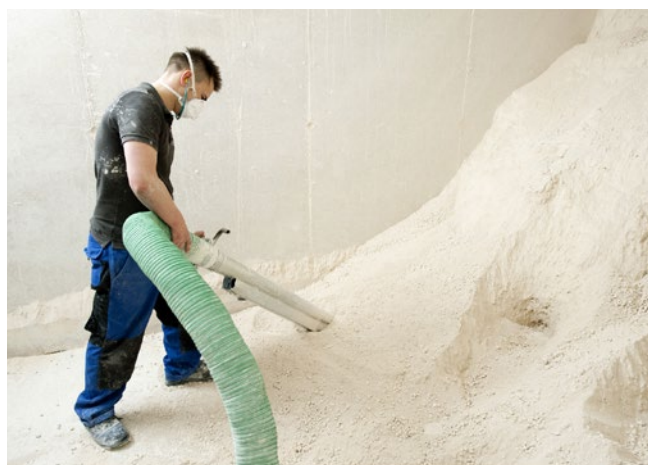
Figure 18: Removal of kaolin from a material box using a suction hose. Source: VBG
