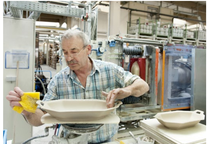
Figure 19: Low-dust moulding of porcelain tableware using the pressure casting method. Source: VBG
