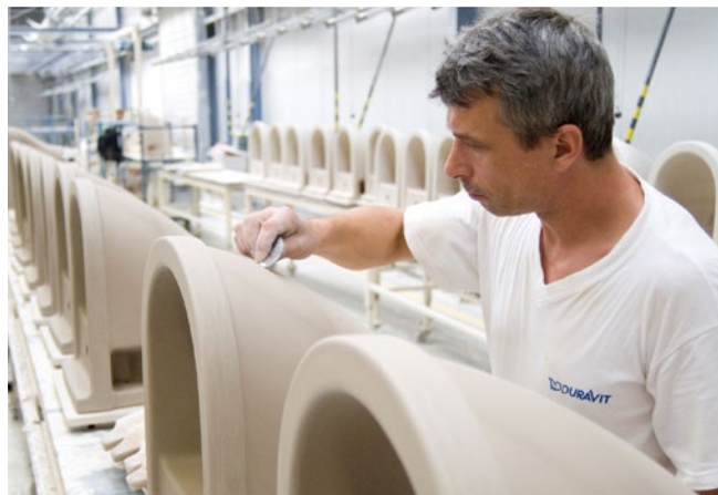
Figure 22: Toilet bowl after moulding. Source: VBG
