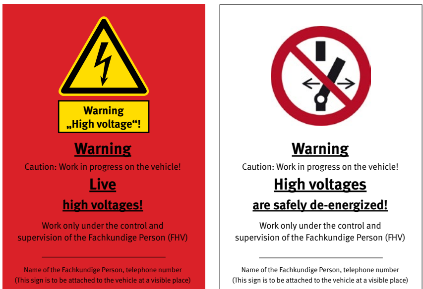
Figure 7 Examples for the marking of HV vehicles in the workshop
