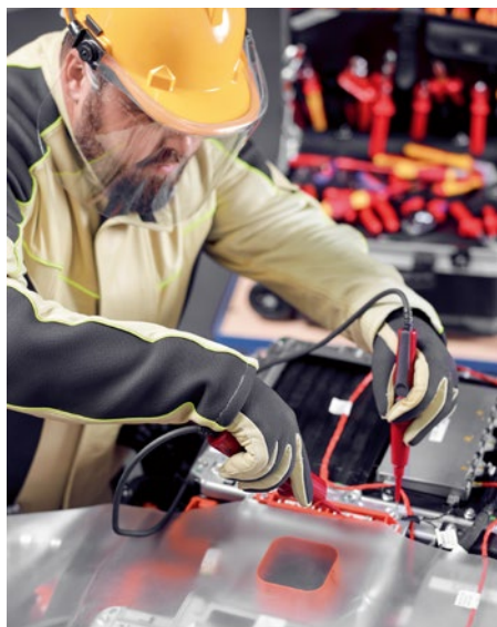
Figure 10 Working on live HV components
