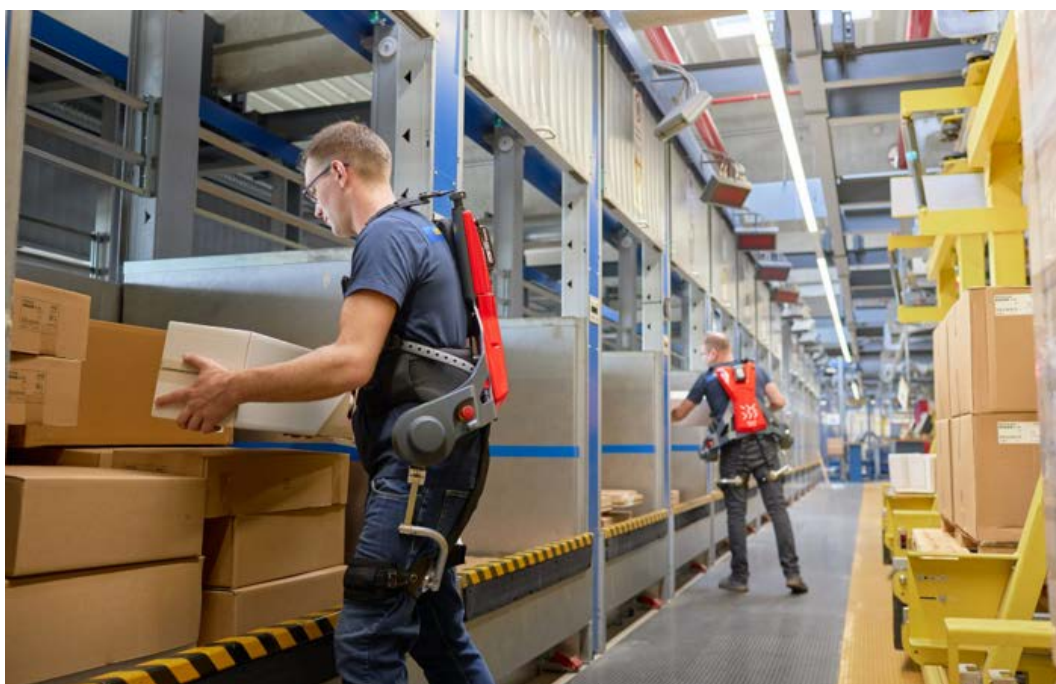
Abbildung 1: Aktives Exoskelett Cray X. Quelle: © German Bionic
