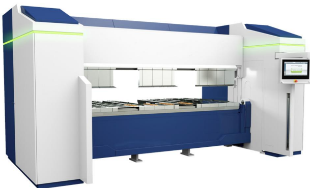
Figure 12 – Example folding machine, front side, safeguarded by a light curtain (green circle)
