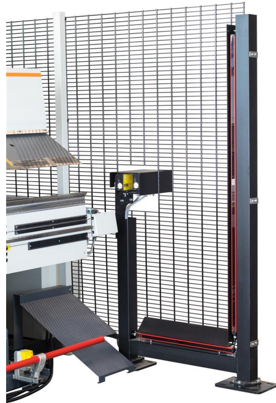
Figure 14 – Example long folding machine as double bend with vertical and horizontal light curtain as access protection and step-behind protection as well as protective fence and laser beams (compare chapter 3.1.4)
