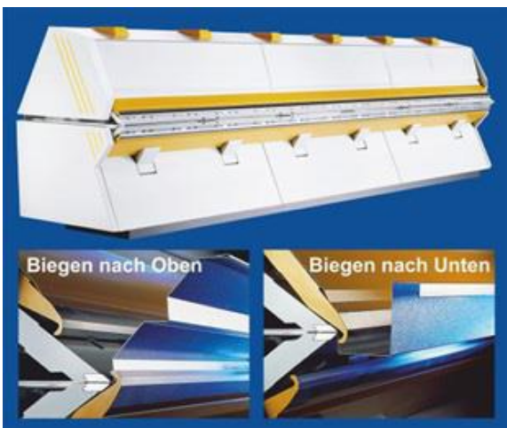
Figure 8 – Example of a long folding machine with two folding beams, i. e. bending upwards and bending downwards
