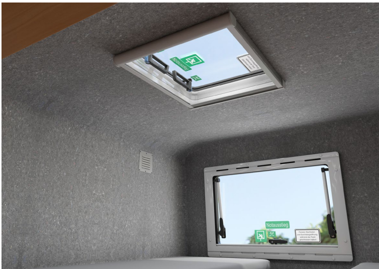
Fig. 10 Second emergency exit in a rooftop sleeper
