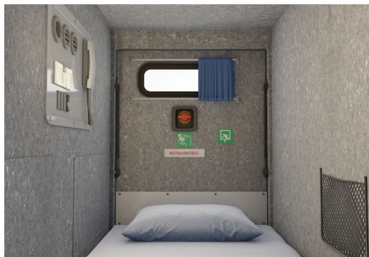
Fig. 13 Emergency exit with window
