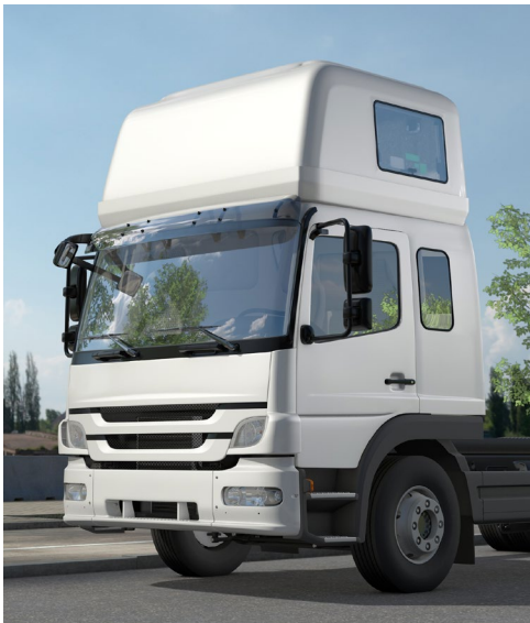
Fig. 1 Rooftop sleeper above a driver's cab
