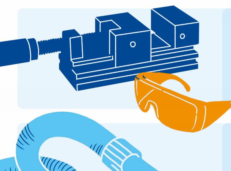
Secure your workpiece against spinning, e.g. using a machine vice. Wear protective goggles.
