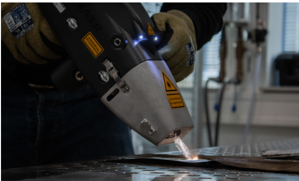
Figure 3 - Laser device with integrated extraction unit
