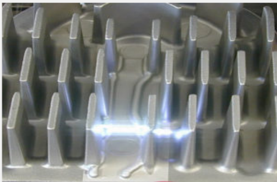
Figure 4 - Laser cleaning on a highly structured component with visible, reflected radiation
