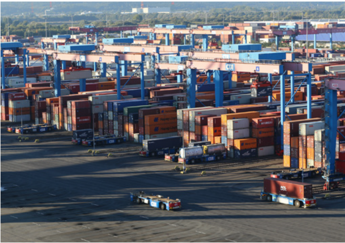
Figure 2 – Container loading with driverless transport systems
