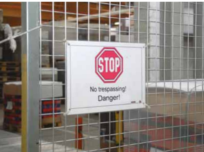
Moving areas of transfer cars with long stopping distances have to be safeguarded, e. g. by safety fences at a height of at least 2 m.
