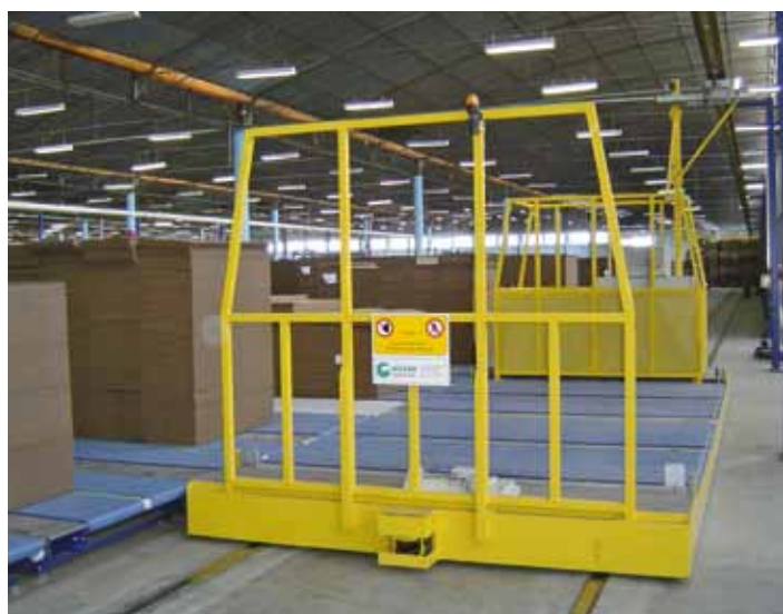
Transfer cars and conveyors are permanently used in the corrugated board industry.
