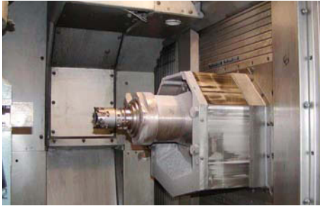
Figure 23 Using gravity for chip removal, steep metal sheet
