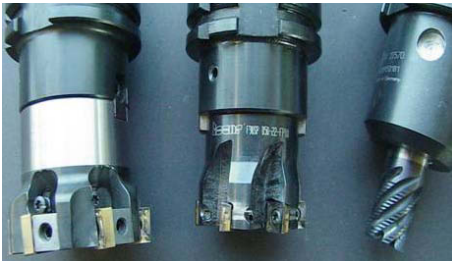
Figure 19 Tools for minimum quantity lubrication
