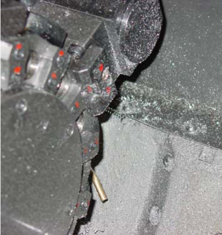
Figure 33 Chip accumulation in corners and edges
