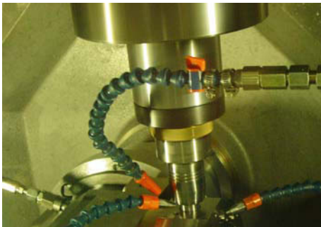
Figure 9 External lubricant feed via nozzles
