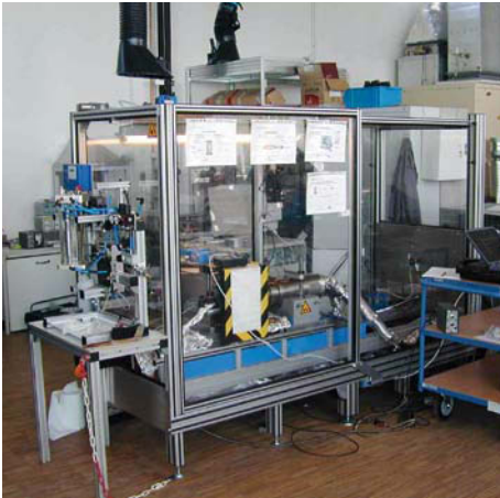
Figure 44 Test bench for determining emissions in the interior
