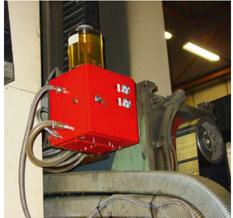
Figure 55 Clean lubricant with MQL system
