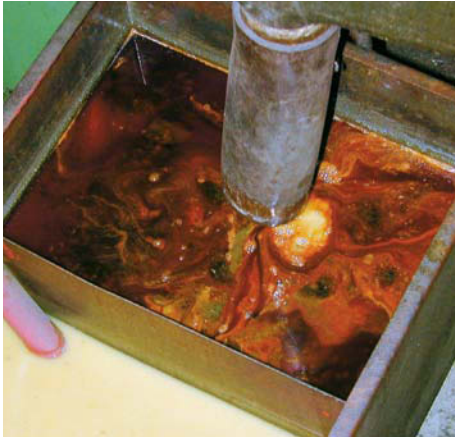
Figure 54 Emulsion in the MWF tank; service life six months
