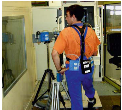
Figure 41 Stationary exposure measurements as well as personal measurements at the control desk
