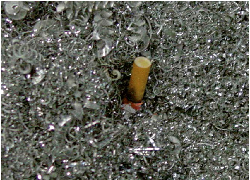
Figure 56 Source of ignition in the chip container
