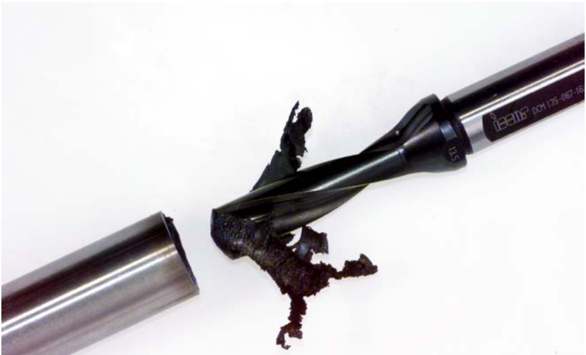
Figure 20 Hot run drill as a source of ignition
