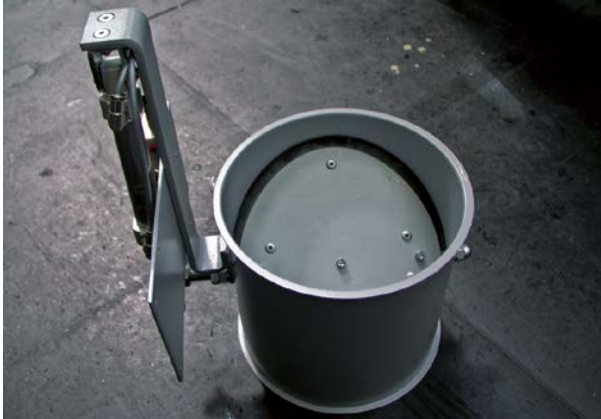
Figure 40 Shut-off valve for ex- tracted air
