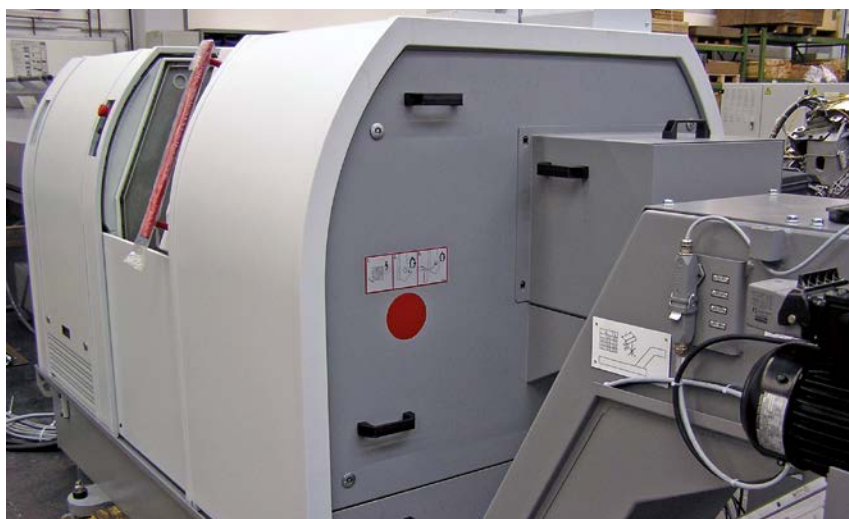
Figure 50 Machine tool extinguishing hole
