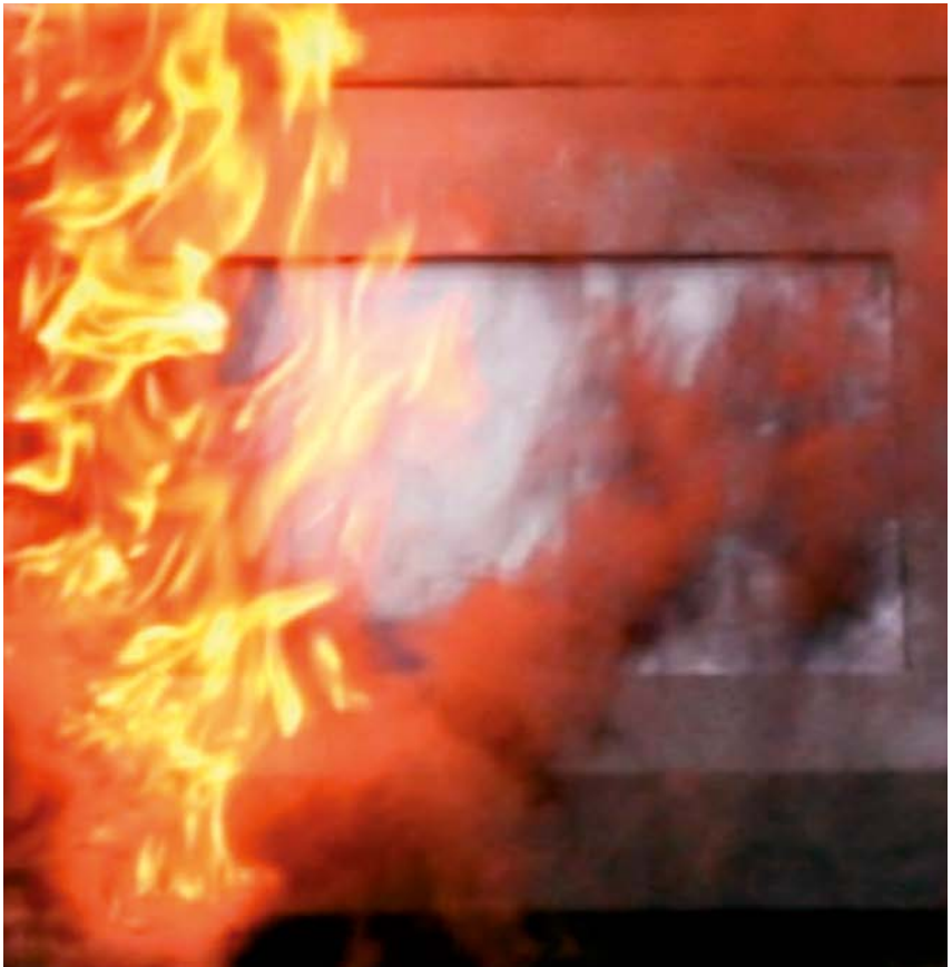
Figure 23 Flame ejection from a door labyrinth
