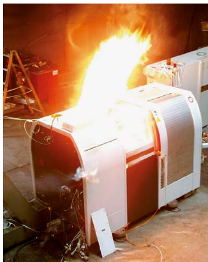
Figure 43 Flame ejection from a pressure relief valve
