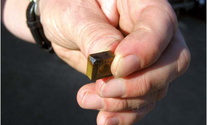
Figure 19 Worn indexable cutting insert
