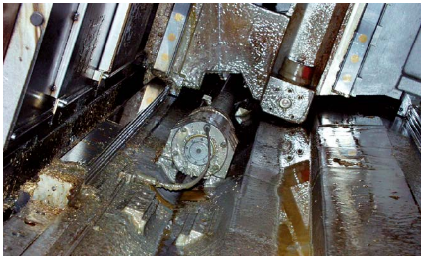
Figure 21 Oil pool formation in the drive room
