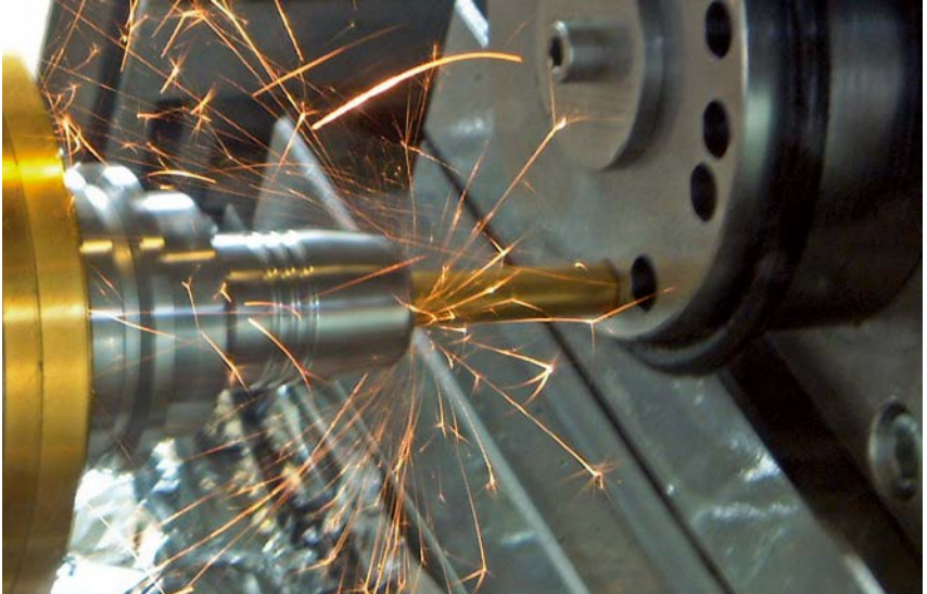
Figure 11 Sparks during drilling
