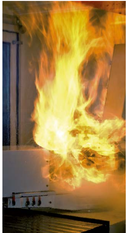
Figure 47 MWF ignition during grinding with subsequent fire
