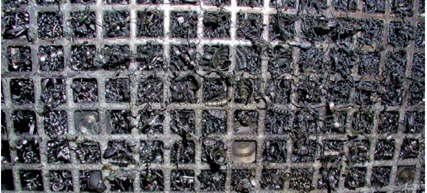
Figure 35 Clogged chip grating
